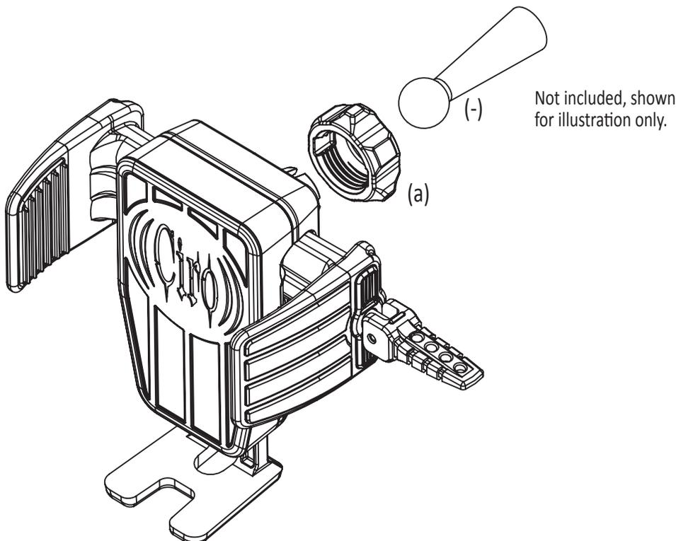
**Cybercharger installation:** *Install the Goldstrike accessory ball mount according to the instructions provided with that product.*
